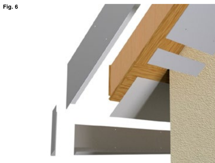
Angled soffit box end construction
